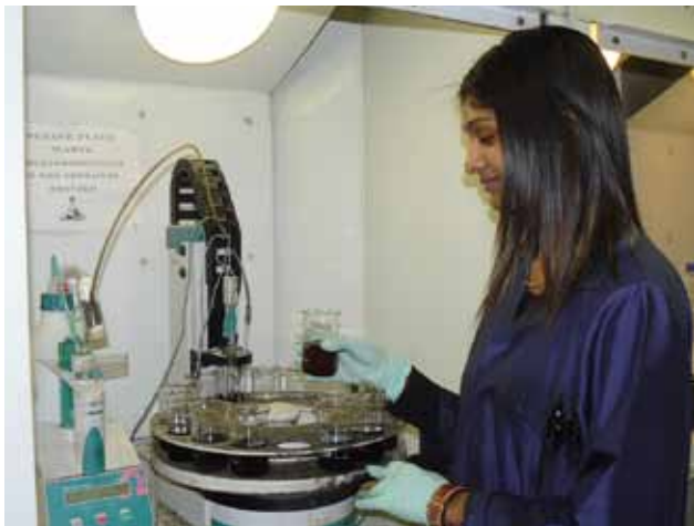
A technician testing oil samples for neutralisation additives
